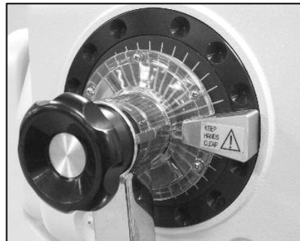
Figure 2.7. Finger Guard Positioned Correctly on Dynamometer for Knee and Hip Attachments.
