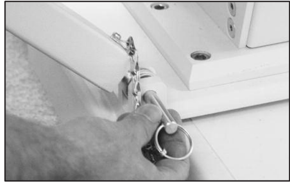
Figure 2.5. Attaching the Seatback Brace to the System 4 Trolley Mount Clevis.
