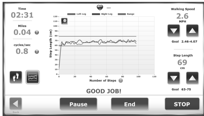
Figure 2.12. Patients Receive Feedback on Step-Length Targets in Histogram View.
