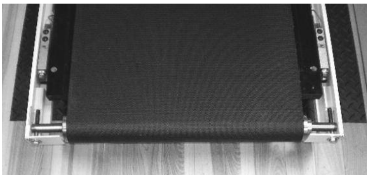
Figure 9.10. Hex bolts shown to adjust belt left or right.
