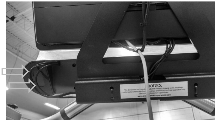
Figure 8.3. The sound bar's power and sound cables (arrows).
