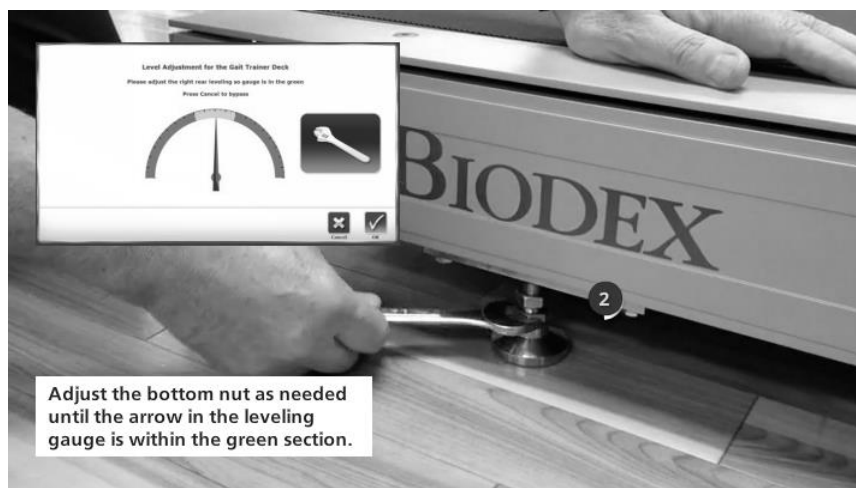
Figure 1.3. Adjust the Bottom Nut
