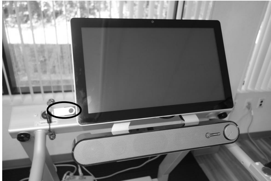
Figure 8.4. USB Port on the Side of the Display with Flash Drive Inserted.
