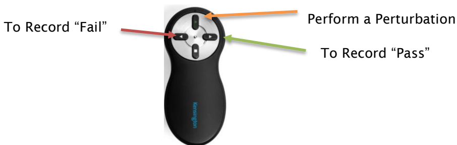
Figure 8.7. Remote Trigger button pre-configuration
