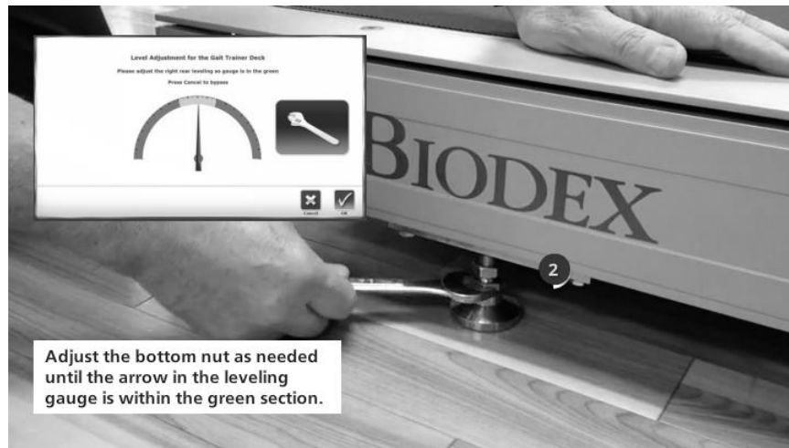
Figure 1.3. Adjust the Bottom Nut
