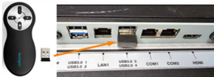
Figure 8.6. USB transceiver connected to the back of display on a USB port.
