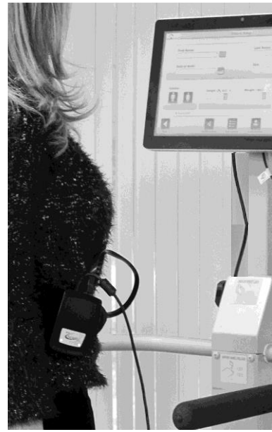
Figure 8.8. Tactile Belt Receiver Boxes can be Charged with a Connection to a Wall Outlet or to the Display on the Device.
