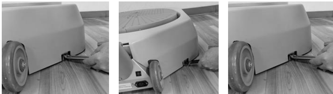
Figure 1.5 Leveling the Base.
