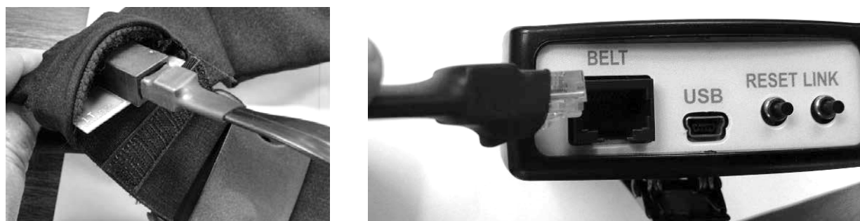
Figure 8.4. Connecting the Tactile Receiver Box to the Belt.
