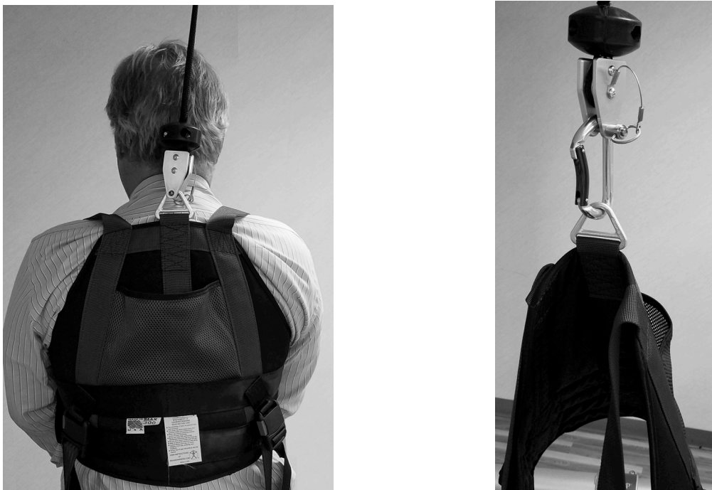
Figure 3.3. Direct Connection to a Single Point Harness.
