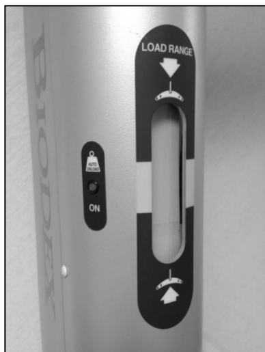
Figure 3.12. The Unweighing Load Range Scale is Located on the Main Column.
