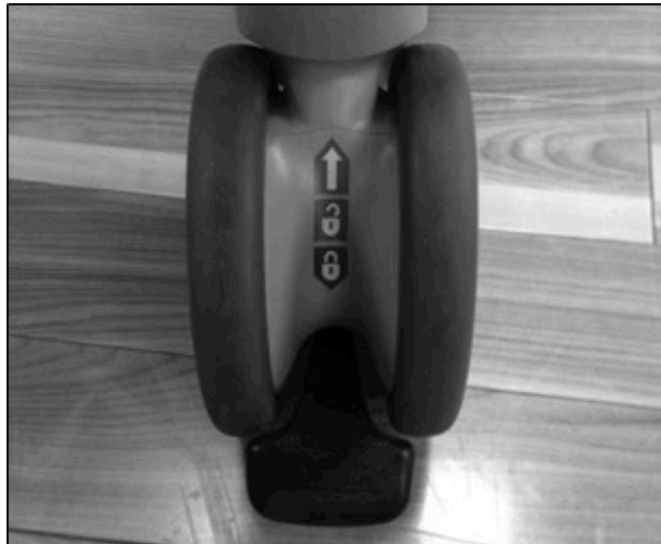
Figure 3.4. The front casters have three settings: completely locked, completely unlocked, and directionally locked.
