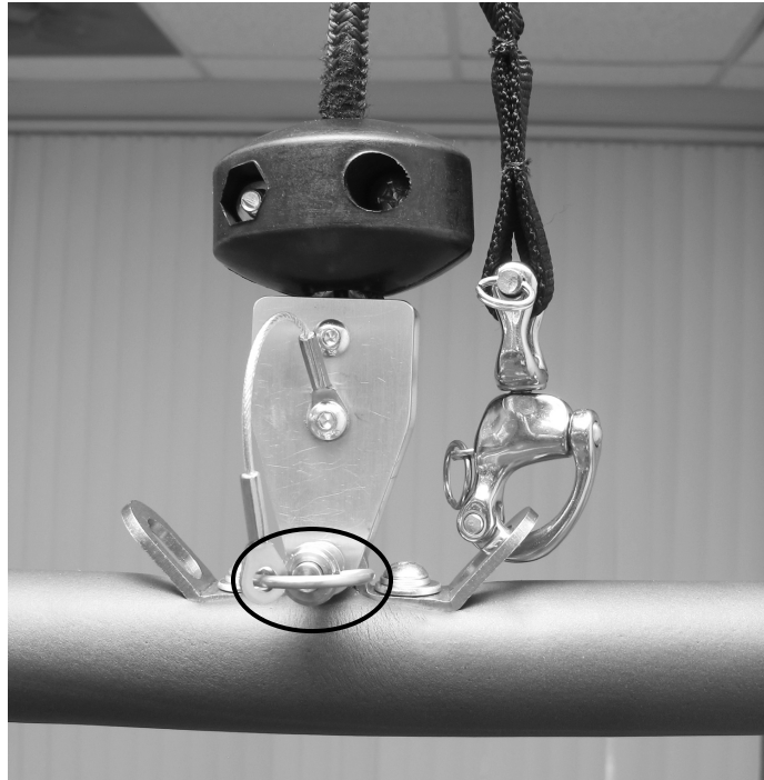
Figure 3.2. Quick Disconnect Apparatus Illustrating Quick Release Pin.
