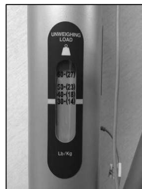
Figure 3.20. Unweighing load scale.
