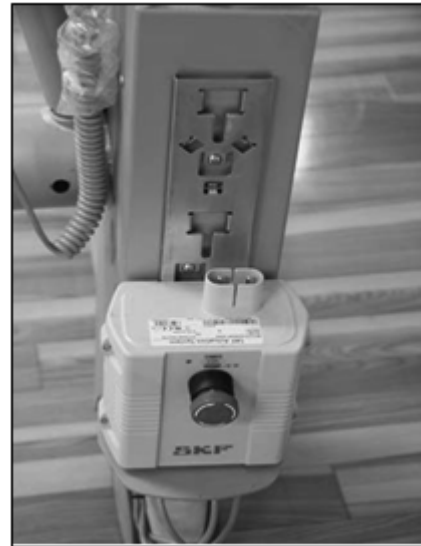
Figure 2.6. The battery pack component fits on top of the base.
