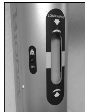
Figure 3.19. The unweighing load range scale is located on the main column.
