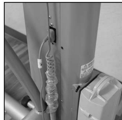
Figure 2.7. The hand-held controller plugs into the main support column.
