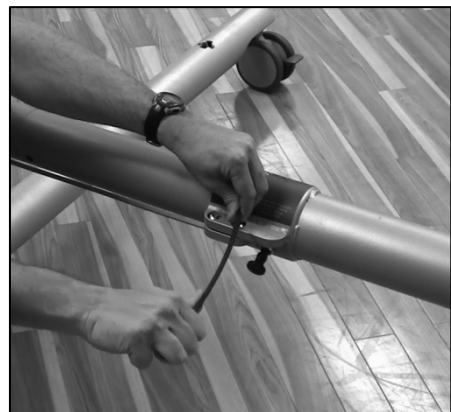
Figure 2.4. The cross tube coupling. Be sure to tighten bolts until Allen wrench bends slightly from torque pressure.
