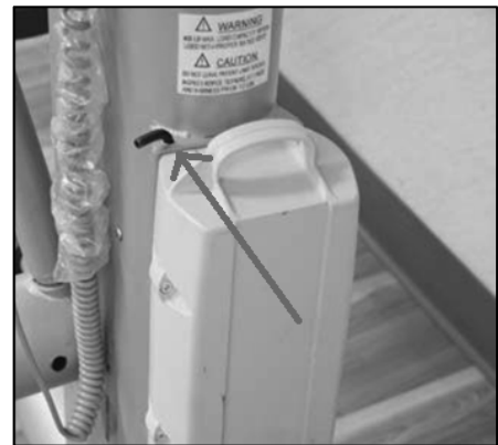
Figure 2.3. The Allen wrench is located alongside the battery pack.
