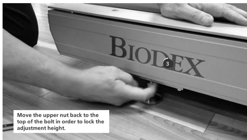
Figure 1.4. Adjusting Gait Trainer Height
