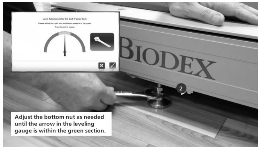
Figure 1.3. Adjust the Bottom Nut
