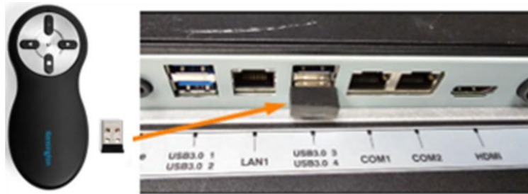
Figure 8.6. USB transceiver connected to any of the USB port on the display.
