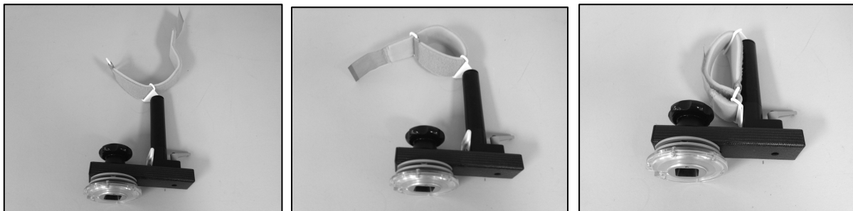
Figure 22. Sequence for threading strap fabric through loop holes
