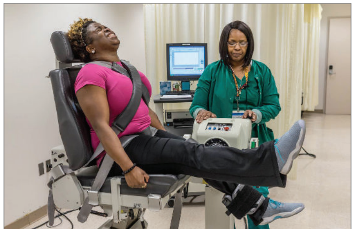
Figure 12. A nurse candidate performs the lower extremity test on one of the Cleveland Clinic's Biodex System 4 Dynamometers. Results are sent to IPCS for interpretation against its massive PCE database.
