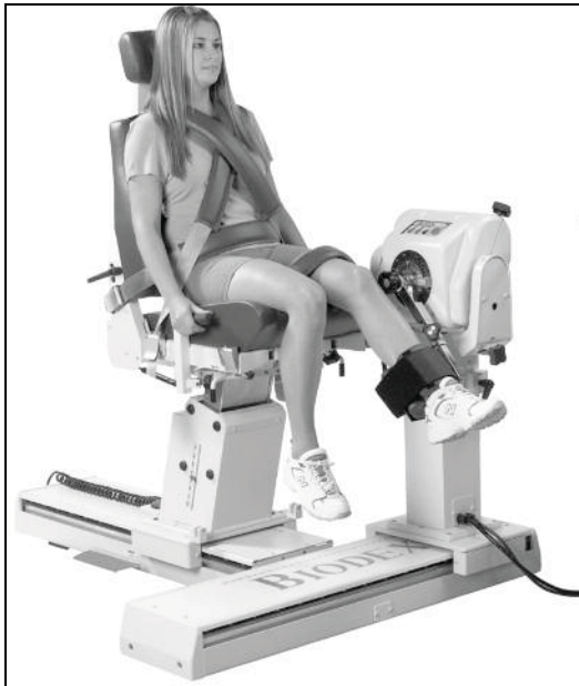
Figure 3.1 Subject positioned for Mixed H/Q Test
