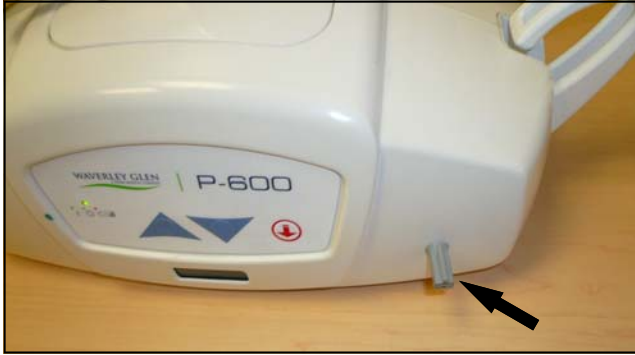
Figure 15A - Gray rubber grommet located on front right side of the lift. Rubber airline is not connected. Note ridge on grommet.
