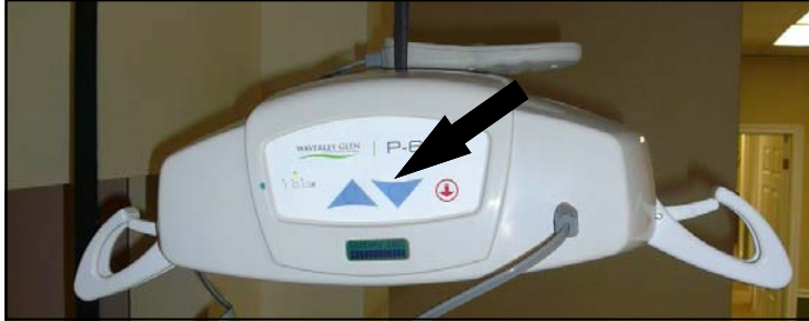
Figure 14A –Lift showing DOWN button located on front right side of lift.
