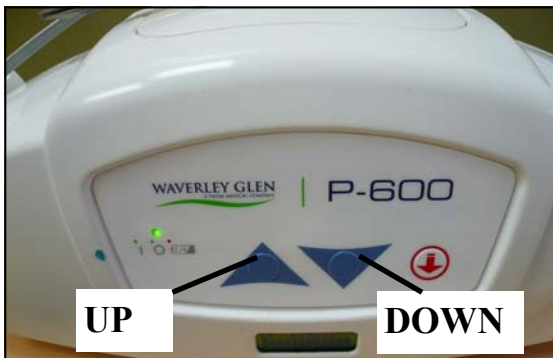
Figure 5C - Front Panel showing raising/lowering buttons
