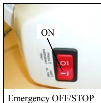
Figure 14D - Close-up of switch ON - Normal lift Operation OFF - Emergency Stop
