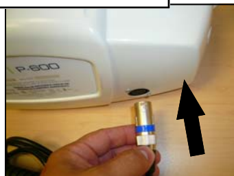
Figure 12D - Connect the charger to the lift. Be sure to line up the 3 metal prongs on the end of the charger with the 3 holes in the black lift "DC" connection.
