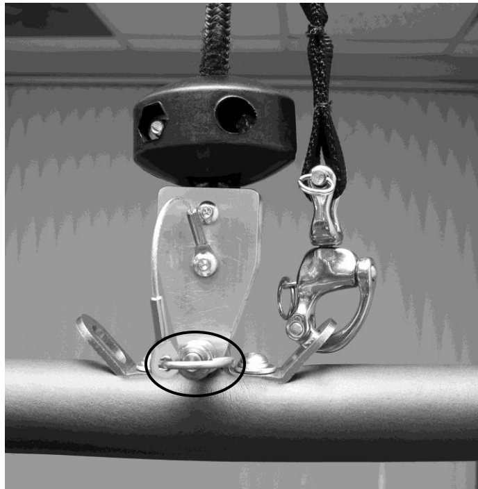
Figure 3.2. Quick Disconnect Apparatus Illustrating Quick Release Pin.
