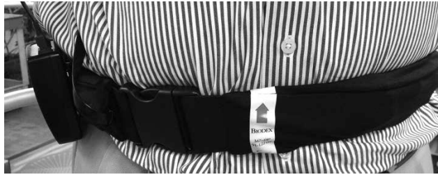
Figure 8.5. Align the Red Arrow on the Tactile Belt with the Patient's Navel.
