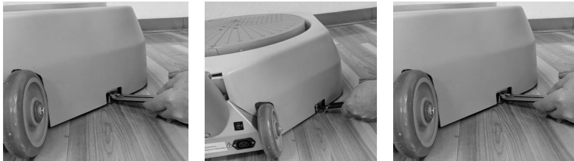
Figure 1.5 Leveling the Base.
