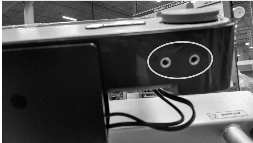
Figure 8.2. The sound bar's headphone and microphone jacks (circled).
