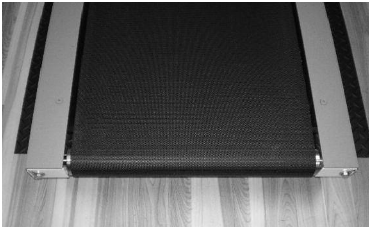
Figure 9.9. Back of Treadmill shown for tensioning bolt location.
