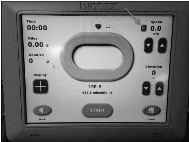
*Figure 3.2 The quick entry keypad is next to the Speed value.*
