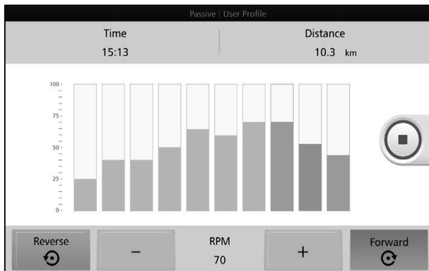
Figure 5.8. Passive User Profile Mode—in-progress exercise screen.
