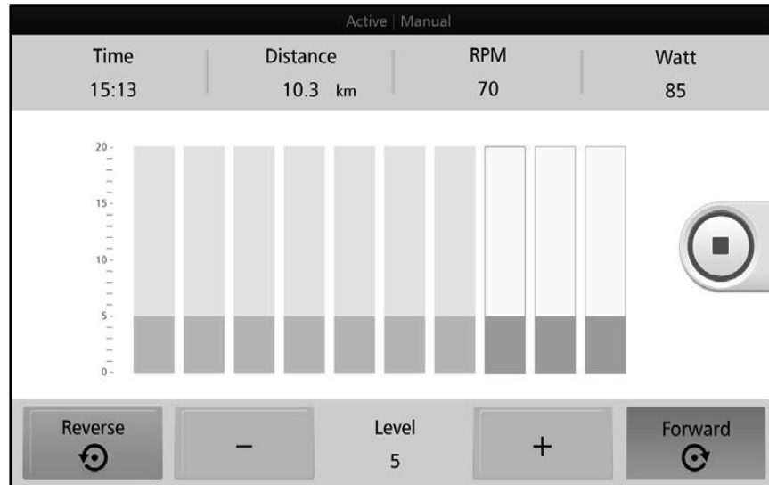
Figure 4.3. Active Manual Settings—resistance levels.
