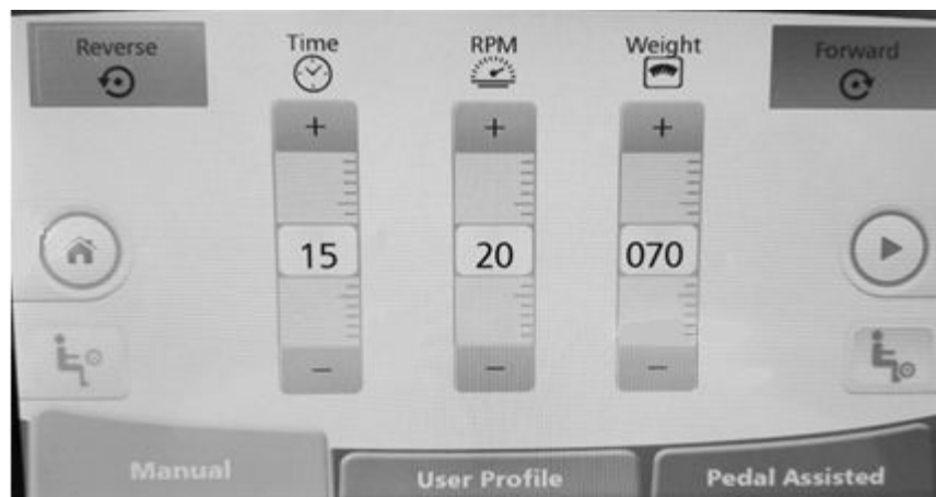
Figure 5.2. Passive Manual Mode—settings screen.
