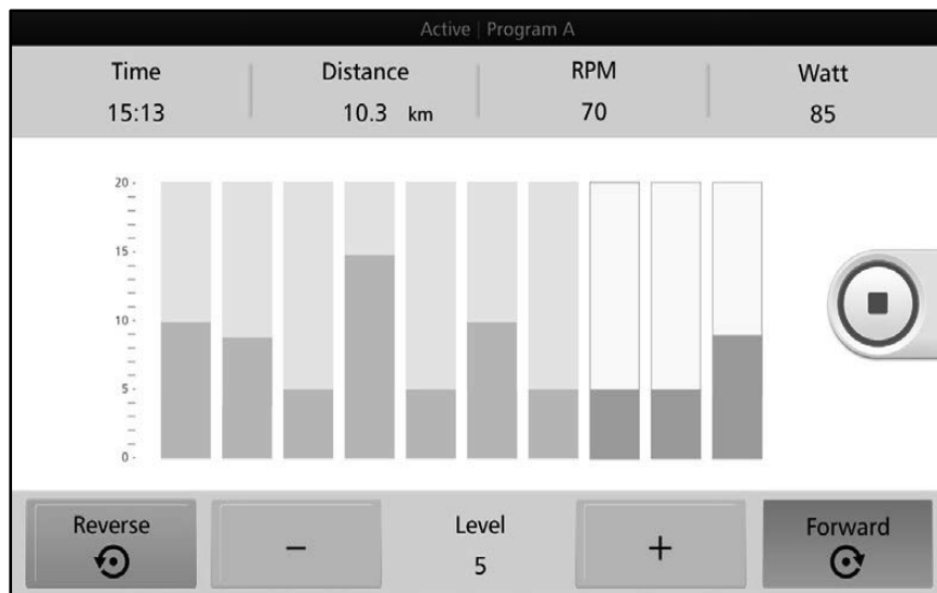
Figure 4.8. Active Resistance Mode (Program A)—resistance level setting screen (individual segments).
