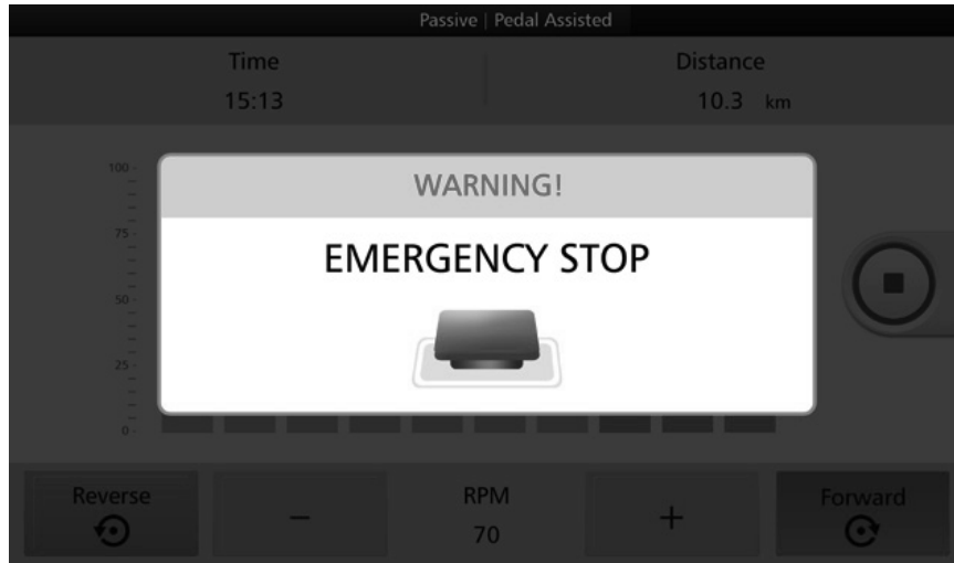
Figure 3.19. Emergency Stop warning screen.
