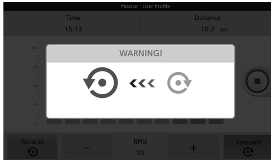
Figure 3.15. Warning screen — Stop pedal/arm cranking completely for a moment before reversing direction.
