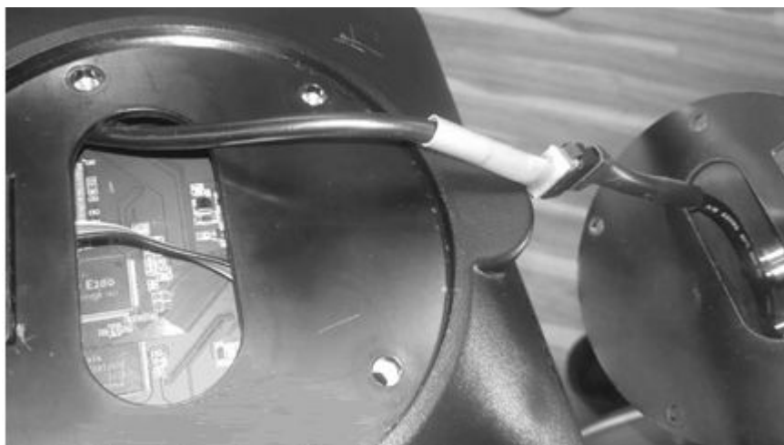
Figure 3.5. Connect the display cable.
