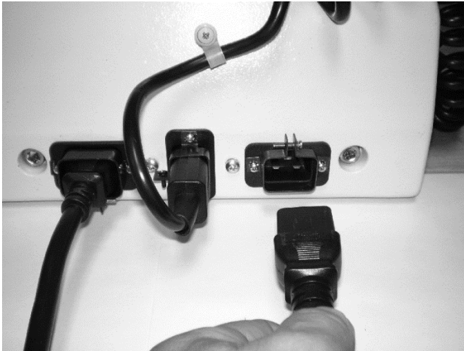
Figure 1.14. Installing the AC Input Cable.
