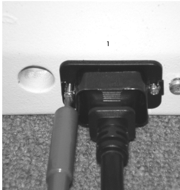
Figure 1.7. Attaching Cable to CDS Cart Power Receptacle.
